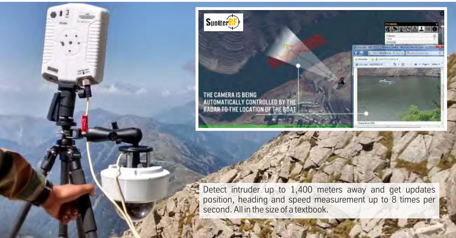
Detect intruder up to 1,400 meters away and get updates position, heading and speed measurement up to 8 times per second. All in the size of a textbook.
