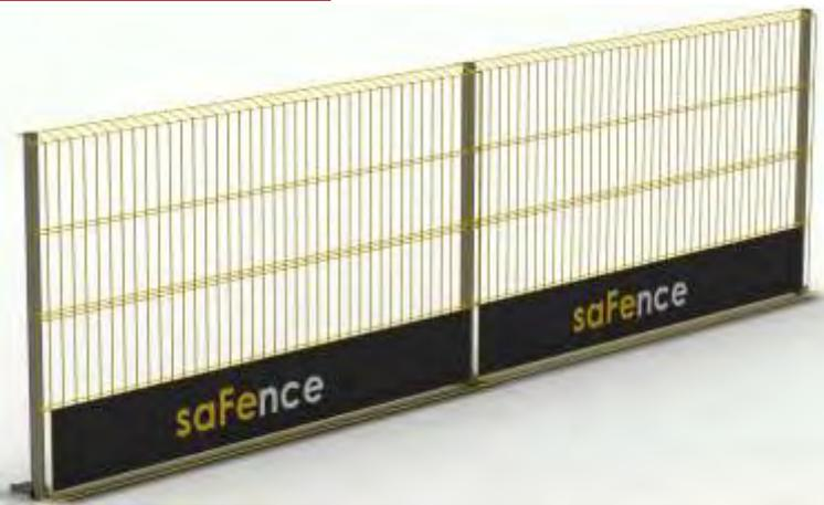
Safence is a modular weldmesh system which is used for fall protection at the edges of construction sites. It incorporates guardrails, toeboards and debris mesh into one single lightweight steel mesh barrier. It has a unique snap and go mechanism which eliminates use of fixtures for installation thus enhancing its ease of usage.
