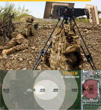
Using Advanced Detection and Classification algorithms, detecting small drones ranges from 200m to 1,000m while immediately cueing cameras to the threat. Using Web based UI (NIO) and video analytics, tighter focus is achieved and false alarms are left almost non-existent.
