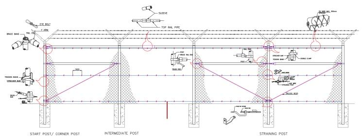
**ELEVATION** of Chain Link Fence System
