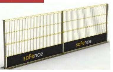
Safence is a modular weldmesh system which is used for fall protection at the edges of construction sites. It incorporates guardrails, toeboards and debris mesh into one single lightweight steel mesh barrier. It has a unique snap and go mechanism which eliminates use of fixtures for installation thus enhancing its ease of usage.
