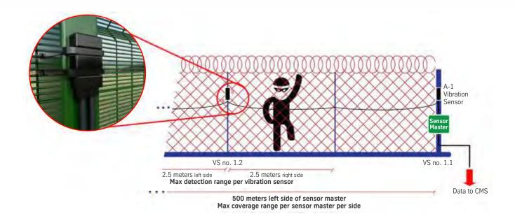
LIMINAL-K (Vibration Sensor) is a fence/wall mounted intrusion detection sensor. It raises an alarm against intrusion attempts like climbing, cutting, breaking etc. by measuring the kinetic energy imparted to the fence/wall.
