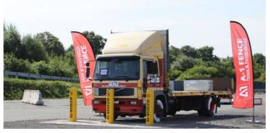
Crash tested for stopping a vehicle of weight **6.8 tonnes** and moving with a velocity of **50 mph** with less than **1 meter penetration**
