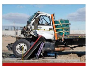
Crash tested for stopping a vehicle of weight **6.8 tonnes** and moving with a velocity of **50 mph** with less than **1 meter penetration**
